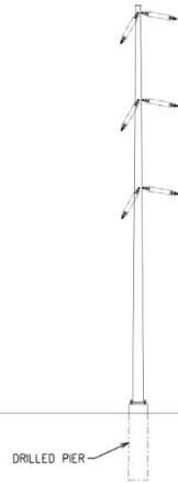
70kV/115kV DVD-3 (TSP)
